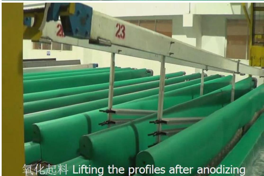
氧化起料 Lifting the profiles after anodizing
