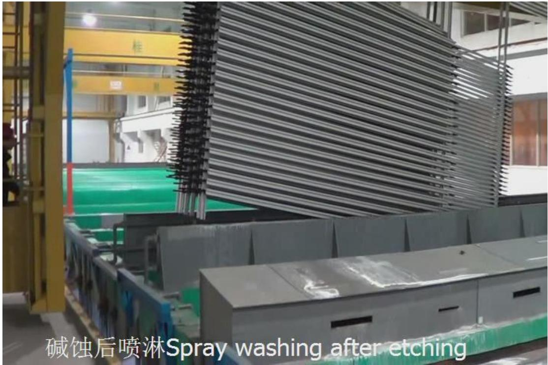
碱蚀后喷淋 Spray washing after etching
